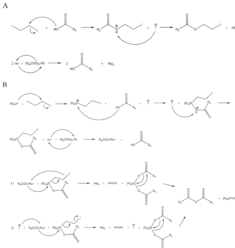
Scheme 1 Proposed mechanism for the synthesis of PbI 2 nanosheets in two steps. (A) describes the slow reaction where TOP is not involved. (B) shows the synthesis after the injection of TOP.
